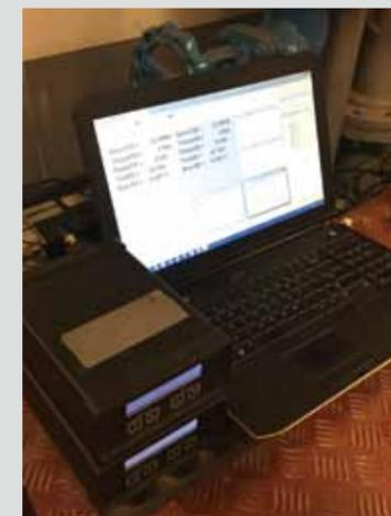
By measuring torsional shaft stresses, we can determine shaft power to verify the engine's rated output. Measuring torsional vibration is also crucial to understanding problems like coupling failures and shaft fractures.
