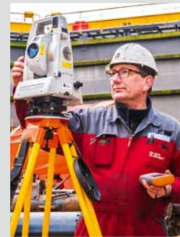
We can measure the geometrical of an object both in itself and in relation to other objects. For example, we can ascertain the flatness of a flange and its exact position and angle in relation to the surrounding structures.
