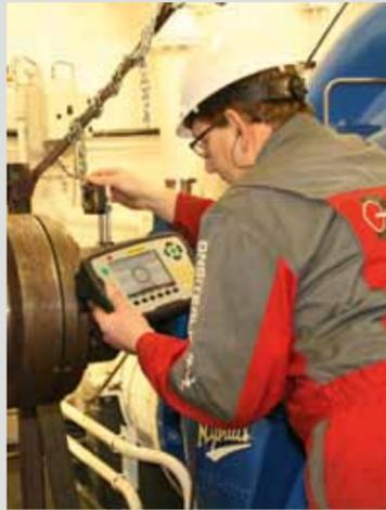
We carry out shaft alignment on all types of rotating equipment, including engines, gearboxes, generators, shaft (support) bearings, pump sets, winches and bow thrusters. We also measure and correct crankshaft web deflection.
